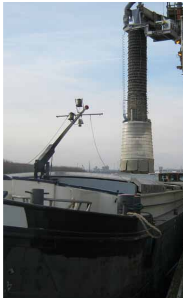
Loading of cement (250 t/h) on barge or tank ships with pneumatically operated sealing cone
