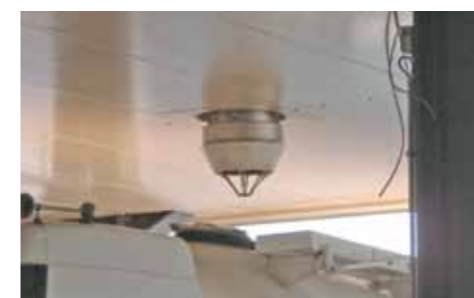
MWV (with docking device, cap lifter, sampler and filter unit for dedusting) for loading of plastic pellets from 44 silos
