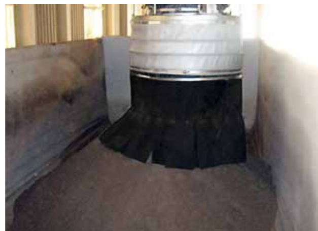
Loading of cement (250 t/h) on barge or tank ships with pneumatically operated sealing cone
