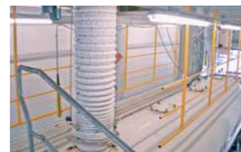
Loading of carbon black in silo truck
